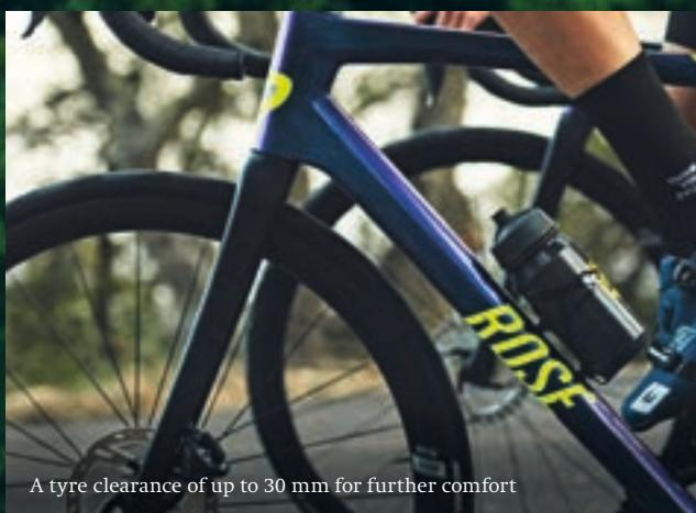
A tyre clearance of up to 30 mm for further comfort
