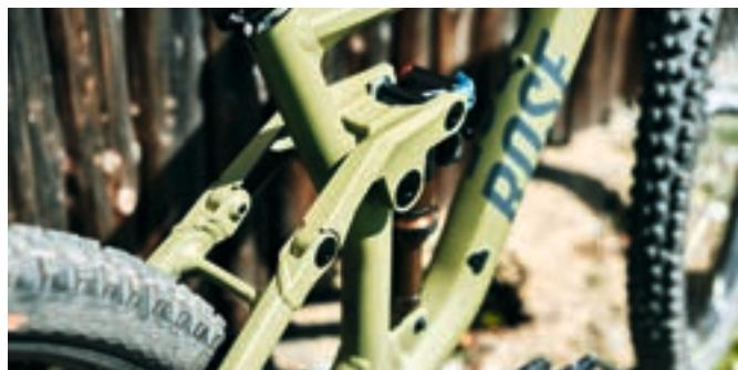
Standing rear shock and trunnion mount: The new rear dropouts design guarantees an especially sensitive response
