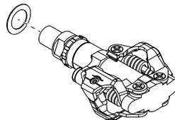
2. Turn the left pedal counter-clockwise to screw it into the thread of the left crank arm and tighten the pedal to a torque of 35 Nm.
