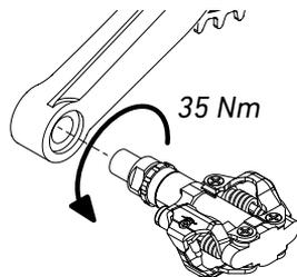
3. Turn the right pedal clockwise to screw it into the thread of the right crank arm and tighten the pedal to a torque of 35 Nm.
