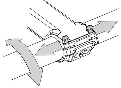
3. First tighten the two lower bolts alternately to a torque of 8 Nm.
