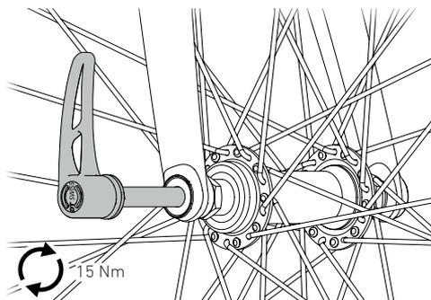
8. Lift the RWS lever (A), turn it to the required position (B) and let go (C).
