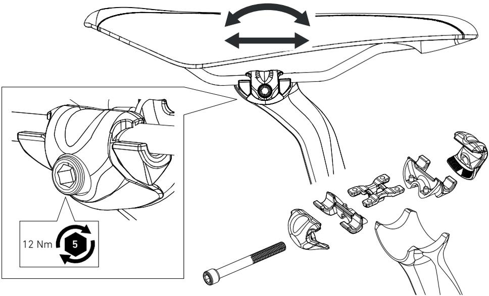
1. Loosen the clamp bolt by about 2 turns. ATTENTION: Do not unscrew the bolt completely!
