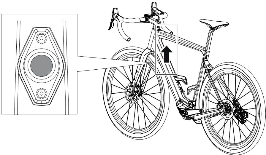
1. Press the on/off button on the underside of the top tube and hold the button down briefly.
