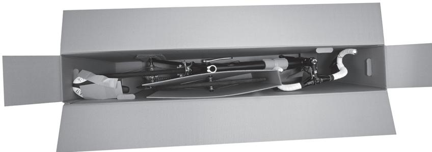
1. Fasten all loose or movable parts or wrap them sufficiently. Sharp or pointed components should be wrapped additionally to make sure they won't damage other parts of your bike and won't tear through the outer packaging.
