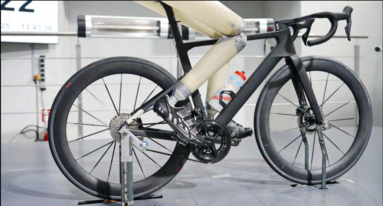
Figure 7: Test setup of the Shave prototype in the GST wind tunnel © Robert Kühnen
